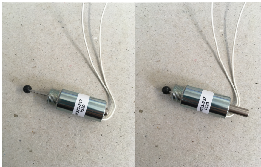
Figure 3.11: Left: Extended solenoid pin. Right: Retracted solenoid.
