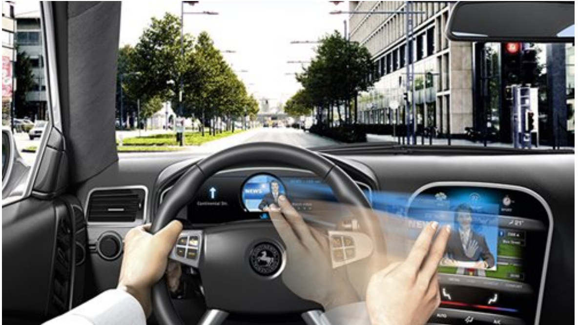
Figure 1.1: Continental's gesture interface [1]. The driver is swiping their hand from left to right to execute a system command.
