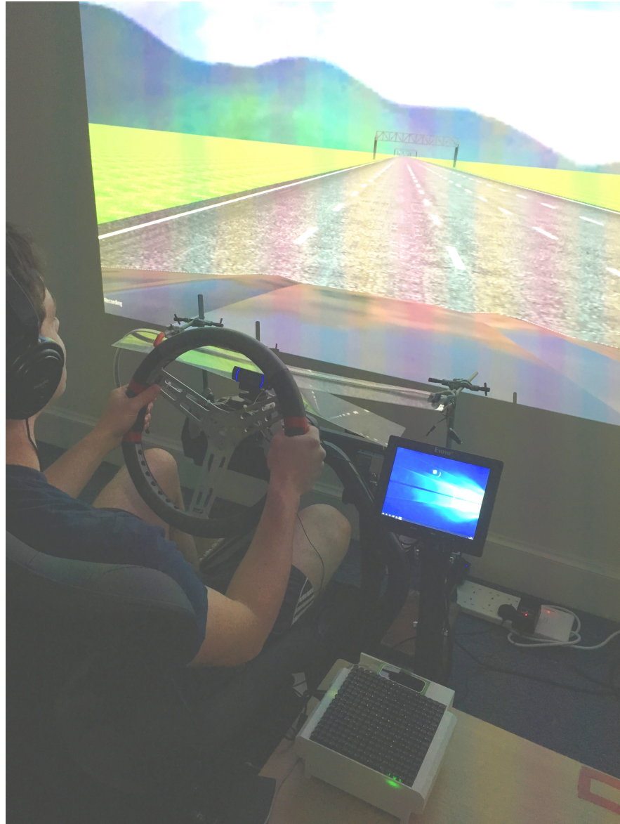
Figure 5.11: Study 7 setup. The Ultrasound array is located to the right of the driver, with the Leap Motion device located next to it. LED strip was placed in front of the driver, the camera recording the driver's eyes on top of the steering wheel base, and the centre console to the right of the driver.
