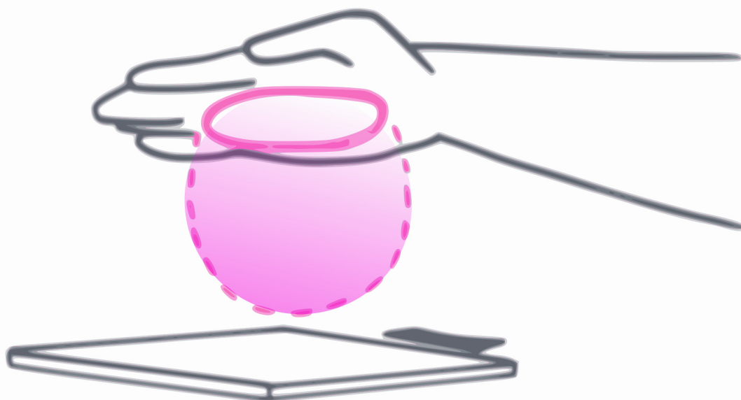
Figure 2.4: Ultrasound creation of a ball in mid-air. The hand passes through the ball and feels its edges. Box at the bottom represents the ultrasound array with 14x14 transducers. Black little box to the right is the Leap motion [4] gesture sensor. In a car, ultrasound feedback would be presented above the area where the gear stick is in front of the centre console.
