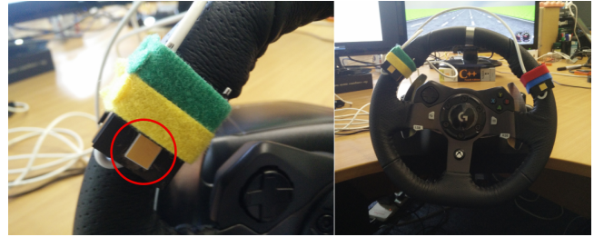
Figure 1: Thermally-enhanced steering wheel with small Peltier elements.
